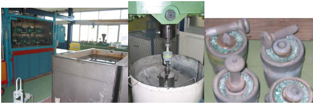
Figure 11 : Residual strength test after thermal cycles on 30 year old HVDC insulators
