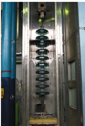
Figure 10 : thermo mechanical test on HVDC Insulators removed after 30 years in service
