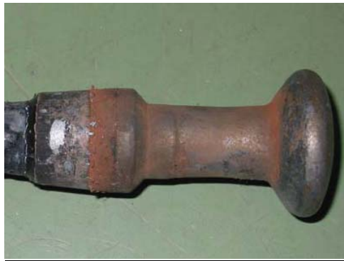
Toughened glass insulators Ref F16P after 25 years at 600kVDC in Itaipu Brazil. (second picture shows effective protection of zinc sleeve on a pin after being removed from an insulator.).
