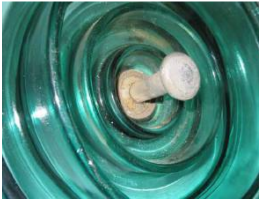
Toughened glass insulators Ref F18P after 30 years at 500kVDC in the USA
