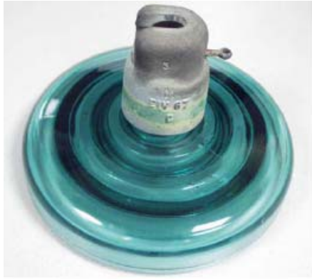
Toughened glass insulators Ref F18P after 30 years at 500kVDC in the USA
