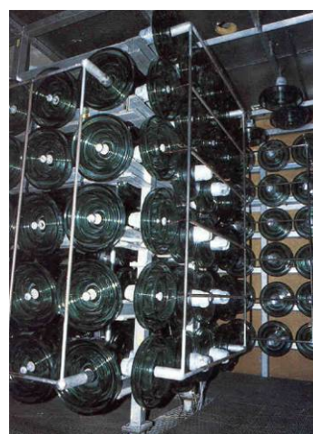
Figure 9 : Ionic migration test chamber
