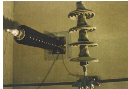
Figure 7: view of fog chamber insulator during the pollution test
