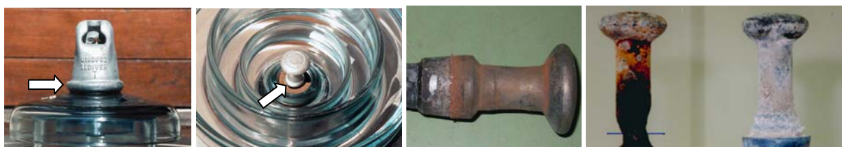
Figure 7 : State of the art HVDC insulator with corrosion protective sacrificial zinc sleeves on cap and pin. Left to right : zinc collar on cap – zinc sleeve on pin side – zinc sleeve on pin from Itaipu 600kVDC after 20 years – difference of behaviour between pin without and with zinc sleeve under extreme pollution.
