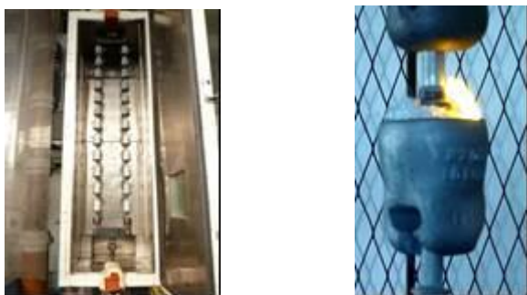
Figure 10 : Left: Thermal mechanical test on stubs. Right: electromechanical test at 70% of rating.
