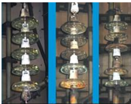
Figure 12: Strings with stubs after power arc testing.
