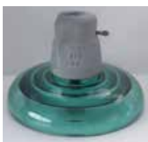
Sediver 210 kN insulator taken from a 500 kV line in Canada after 45 years in service
