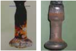
Corroded pin without zinc sleeve Pin with zinc sleeve
