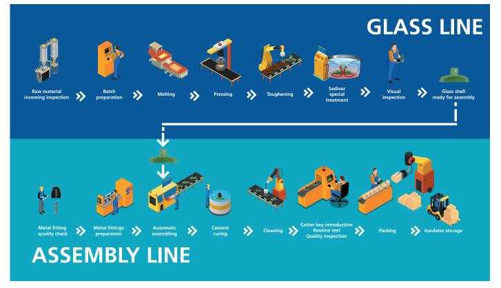
Shanghai factory which started operation in 2004, has one furnace and two lines of production with a monthly capacity of approx.2330 tons of glass, with the following process
