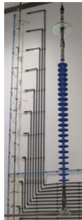
Figure 13: Silicone coated glass string (top) with no activity and equivalent polymer insulator (bottom) during a salt fog preconditioning test at -200kVDC at 20g/l with dry band activity leading to flashover of the polymer insulator after approximately 1h.
