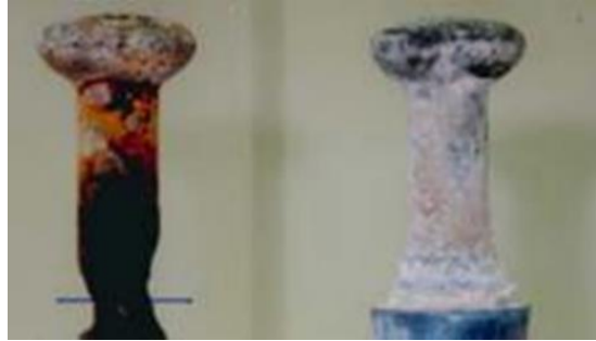
Figure 3: Benefit of a DC zinc sleeve on the pin of a DC insulator. Left without and right with a zinc sleeve after approximately 15 years in a very challenging coastal environment.
