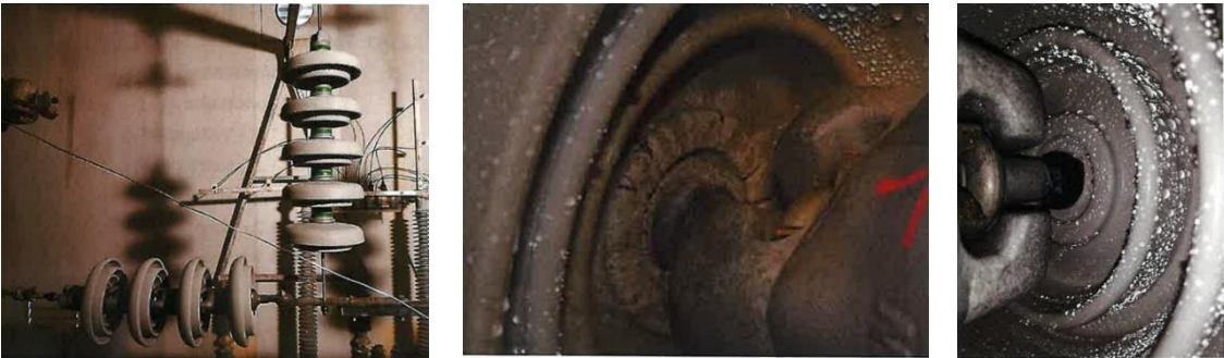
Figure 11: 2000 h multi stress test with a DC applied voltage. Center Type A with erosion and hydrophobicity HC5-6. Right Type B no erosion and HC1-2.
