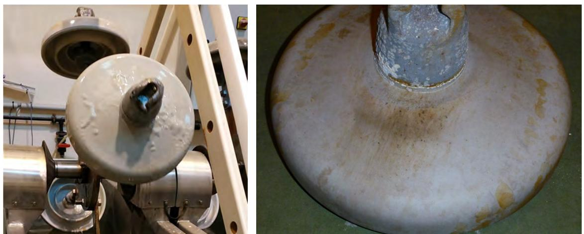
**Figure 13:** Loss of adherence of silicone type B after 28000 cycles on glass Insulator (left). The same Insulator 24h after the end of more than twice the test duration (65000 cycles)
