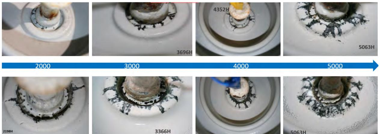
**Figure 3:** evolution of erosion of the coating on glass insulators in a 5000h multi stress test
