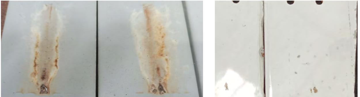
**Figure 8 :** Typical results of the inclined plan test at 3.5kV. All samples are eroded (left) through their thickness with a mark on the tile underneath but without a destruction of the tile itself (right)
