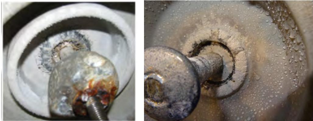
**Figure 2:** Erosion on 2 different coatings in a 1000h salt fog test with a USCD=25mm/kV
