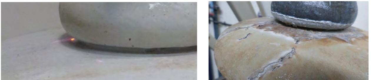
Figure 14 : Electric activity on porcelain after approximately 7000 cycles (left) and erosion as of approximately 13000 cycles on porcelain with type A silicone.
