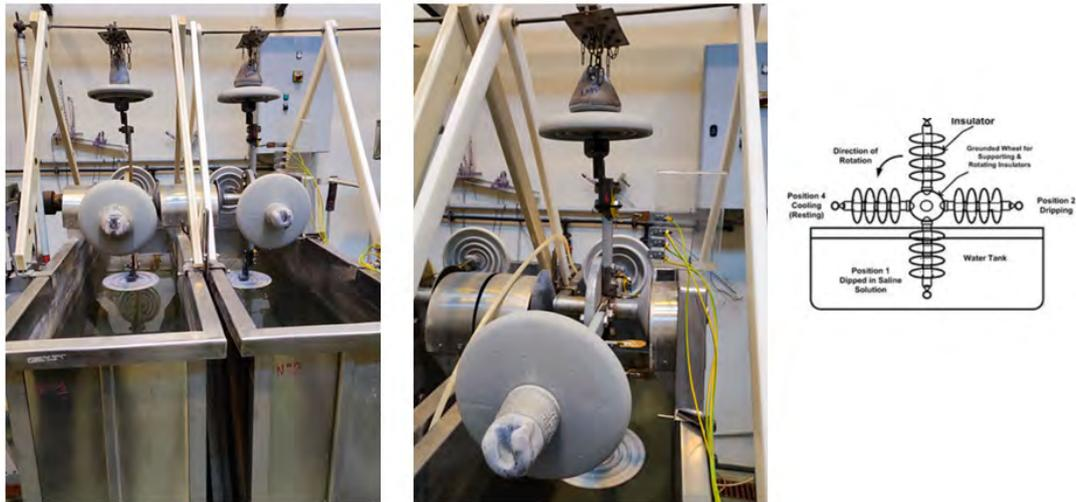
**Figure 11:** Set up of the tracking wheel test as per IEC 62217 (right) and actual arrangement in Sediver R&D laboratory with silicone coated glass and porcelain insulators
