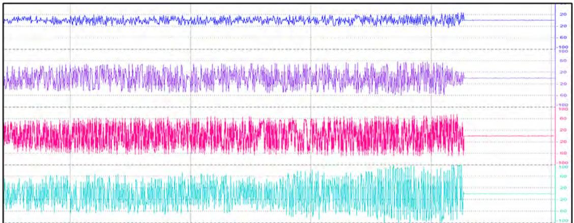
Figure 17 left: from top to bottom: Glass with silicone type B, Porcelain with silicone type B, Glass with silicone type A, Porcelain with silicone type A. Readings at approx. 7000 cycles.
