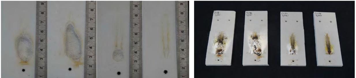
**Figure 10:** Result at 3.5kV showing a coating which pass (left) and one which failed (right)
