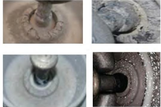
**Figure 6** : Typical results showing erosion among coating chemistries
