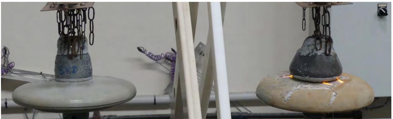
Figure 15: Comparison of dry band arcing activity at the base of the cap of Sediver glass having a flock at the base of the cap and a porcelain insulator. (Silicone type A at 10000 cycles).
