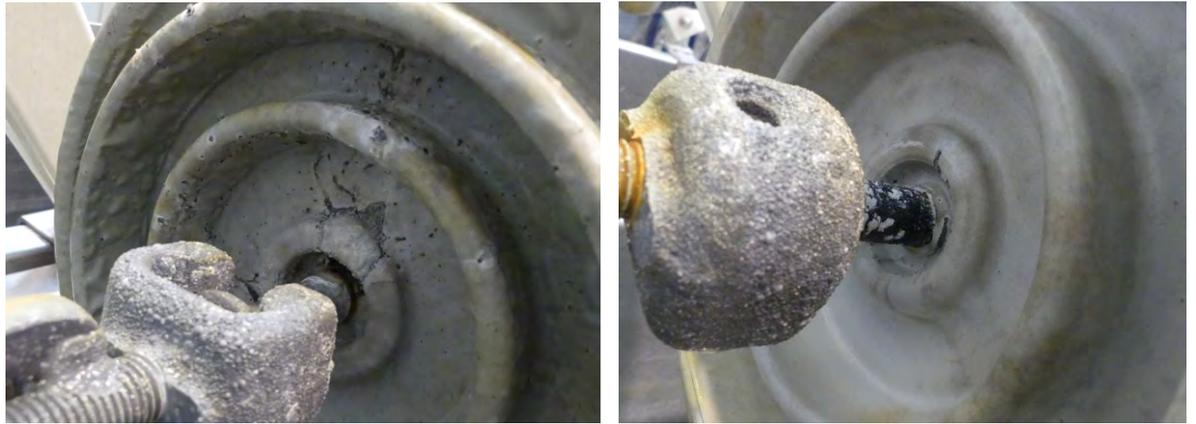
Figure 16: Glass insulator at approx. 20000 cycles. Left silicone coating type A, Right Silicone coating type B
