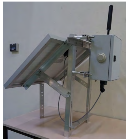
Figure14: Smart E leakage current monitoring system
