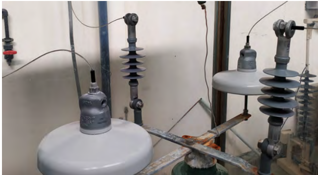
Figure 13: difference of leakage current between a silicone coated glass insulator and a DC polymer. 20g/l with samples at 30mm/kV. Applied voltage 15kV.
